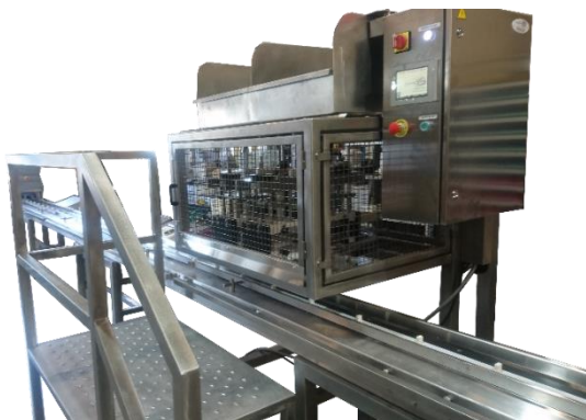
Semi-automatic pocket filler Bi-products : dosing 2 products at once
